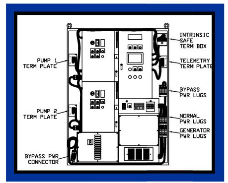
Field connections are limited to terminations in the side compartments. This reduces the risk of jobsite debris entering the areas with sensitive components.
